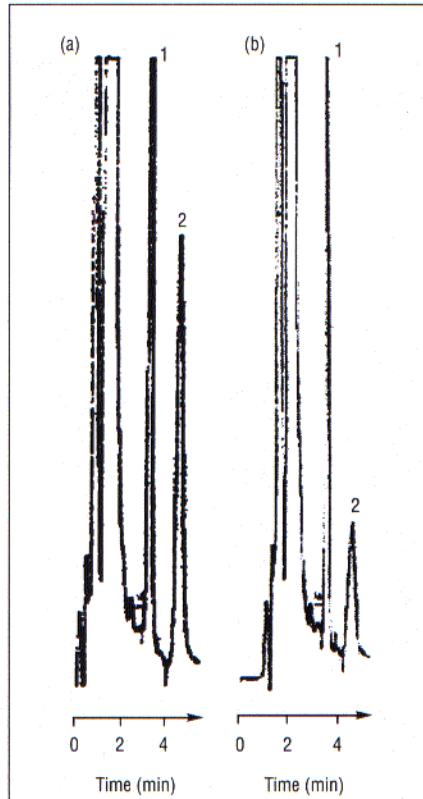
**FIGURE 1:** Injection of (a) calibration standard and (b) internal standard spiked into a normal urine sample. Sample volume: 20  $\mu$ L. Other conditions are described in the text. Peaks: 1 = internal standard, 2 = dabsyl-hydroxyproline.
