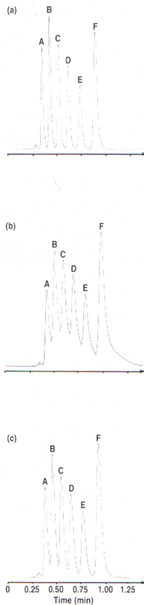
**FIGURE 1:** Chromatograms from a  $3 \times 3$  column used in (a) a standard LC system with an 8- $\mu\text{L}$  detector flow cell; (b) the same system as (a), but with 20 cm of 0.046-in. i.d. tubing connecting injector and column; (c) the same system as (a), but with poorly assembled fittings at inlet and outlet of system. Other conditions given in text. Peaks: A = benzene, B = toluene, C = ethylbenzene, D = isopropylbenzene, E = *t*-butylbenzene, F = anthracene.
