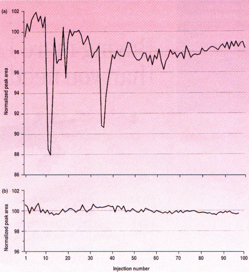
**FIGURE 1:** Plots of normalized peak area vs injection number for 100 consecutive injections (a) before and (b) after degassing the autosampler wash solvent and purging. The plots have been corrected for drift. See text for details.
